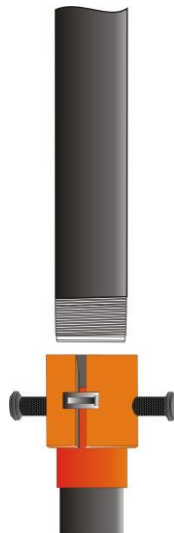
Figure 5 – Make-up with special bell guide
