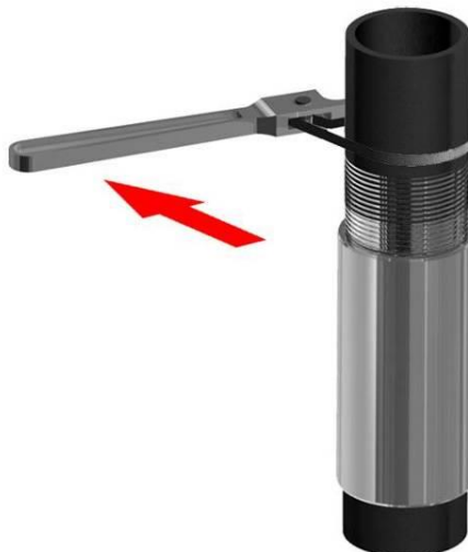
Figure 10 – Make-up start with strap tongs
